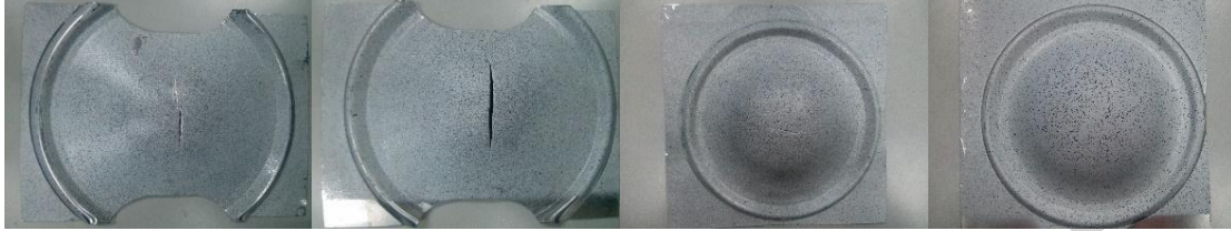
Fig. 8. Bulge test parts: (a) AA1100 plane-strain; (b) AA5052 plane-strain; (c) AA1100 equibiaxial stretching; (d) AA5052 equibiaxial stretching
