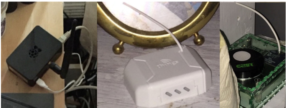
Figure 1. Hub (left), temperature/humidity sensor (middle) CO 2 sensor (right) deployed in situ.
