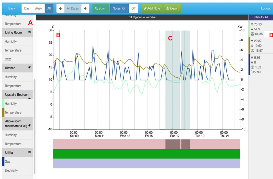
Figure 2. The interactive web app enables (a) filtering (show/hide) of sensor data sources, (b) pan and zoom time series line charts, (c) annotations (highlights) viewable on click, and (d) stats for selected sources (min/max, average, cost in £).
