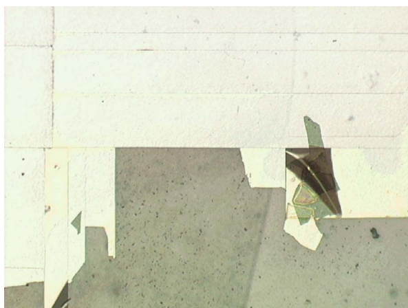
Fig. 2.. A thin zinc-blende GaN layer mounted on glass after removing the GaAs substrate [35].
