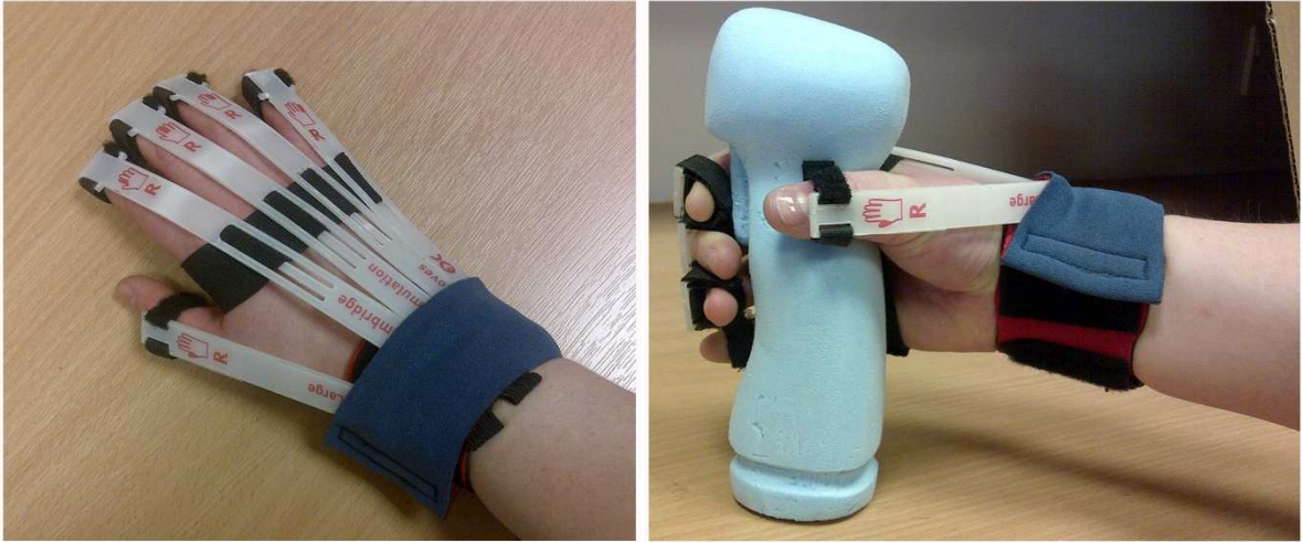
Figure 6. Simulation Gloves- The specifically designed gloves restricted movement in the hand fingers and wrist, allowing empathy with the elderly demographic.
