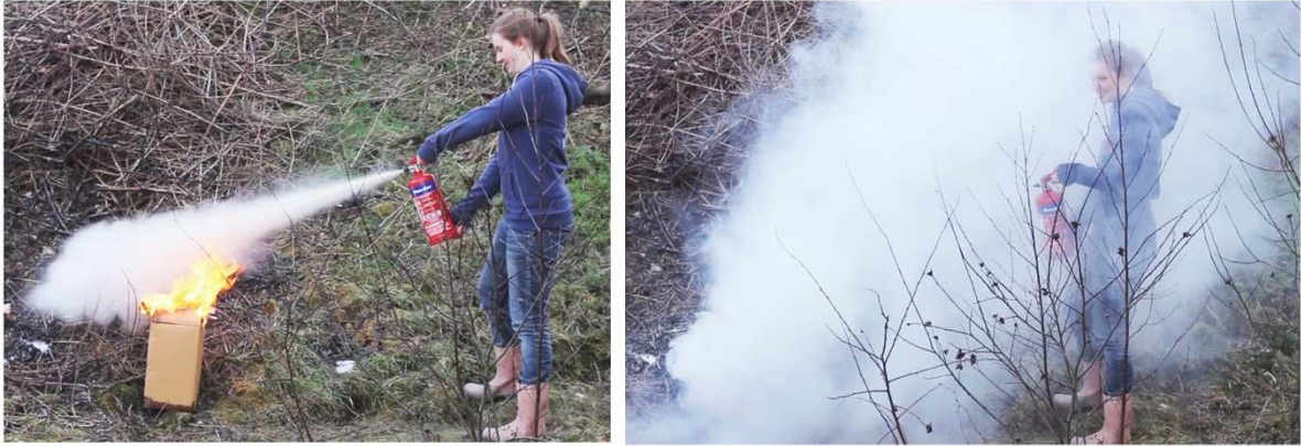
Figure 1. Product Evaluation- the extinguisher was more powerful than expected, and produced clouds of powder obscuring the participant's vision.
