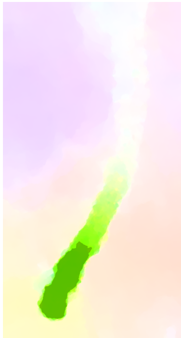
(c) Coloured Optical Flow between Frame 176 and 177 Frames. The brightest region green region has a maximum velocity.
