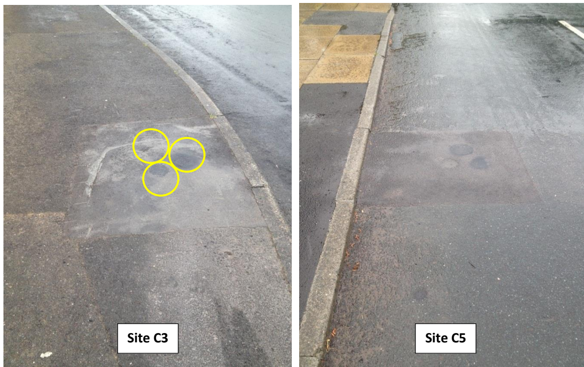
Figure 2: Location of three cores taken by Lab A, Lab B and Lab C from site C3 and C5
