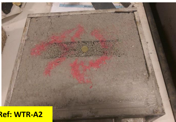
Figure 7: Specimen extraction and testing in wheel tracking apparatus
