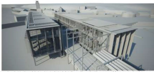
rendered virtual model showing technical detailing with vertical louvers and feature steelwork trusses
