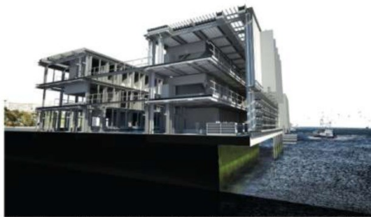
design section created from 'sliced' virtual model with post image editing showing context & materials
