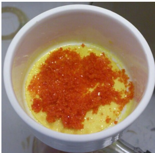
Figure 5.4: Recovery of the orange crystals of PIH by vacuum filtration for use in the ISIS experiment.
