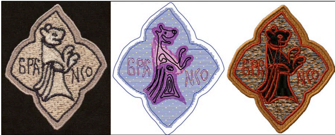
Bear Antenna from the Branko Belt Project. Left: finished textile antenna; Center: assignment of laying stitches for conductive silver thread; Right: assignment of decorative embroidery stitches.
