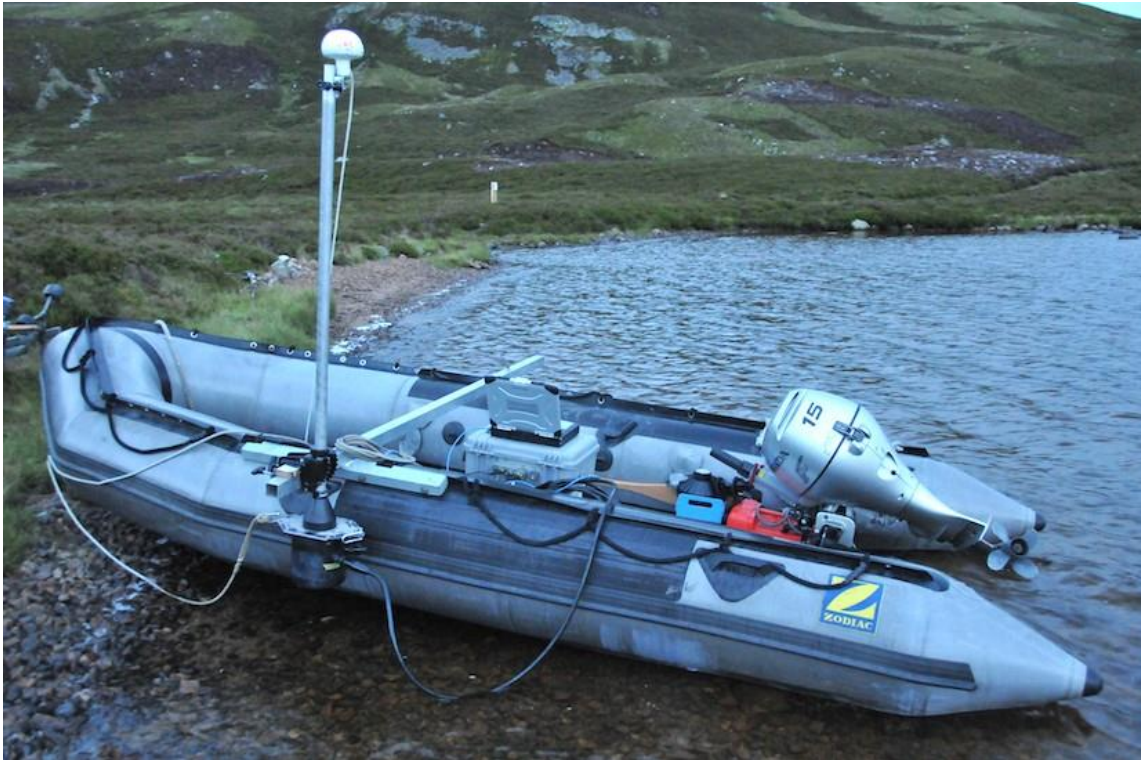
Figure 8. A hydroacoustics system deployed on a 4.8 m RIB. Sound is projected and recorded by a transducer mounted on a vertical pole to the side of the vessel, with a GPS receiver mounted at its top to provide positional information. The system's surface unit is visible as a grey case in the centre of the vessel, with a controlling laptop computer on top of it. The system is powered by a single 12 V battery visible in a blue casing towards the stern of the vessel. © Ian Winfield.
