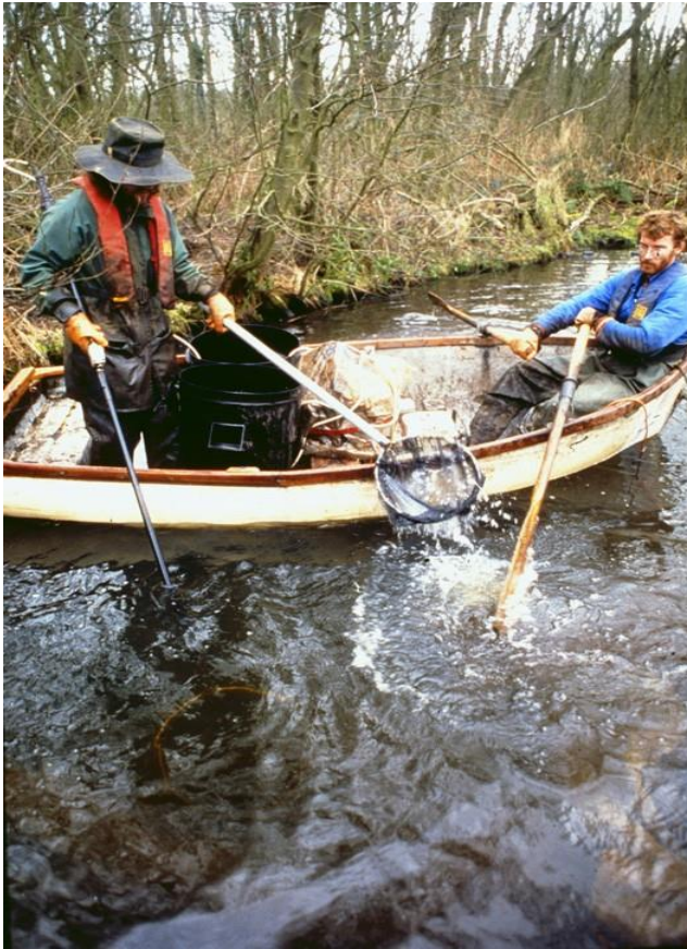
Figure 5. Example of a suitable boat and setup for PASE with the boat controlled by push-rowing and the operator in sight of the oarsperson at all times for safety reasons. © Jane Madgwick Broads Authority.
