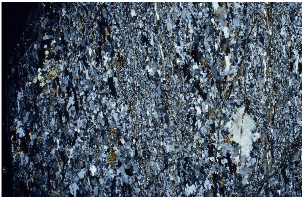
Figure 406. Mylonite (S73582) thin section under XPL. Contains British Geological Survey materials © NERC 2016. No scale available
