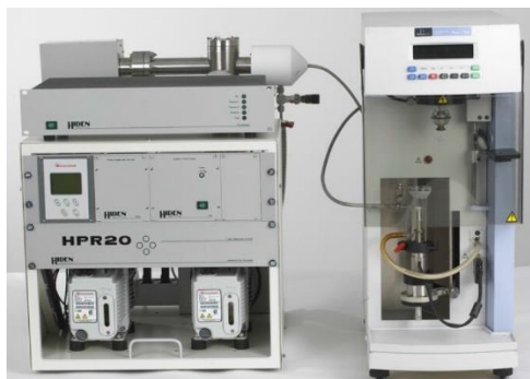
Figure L.4 Pyris 1 TGA (left) coupled to a Hiden HPR20 mass spectrometer (right) via a ceramic-walled heated transfer line (manufacturer supplied image).
