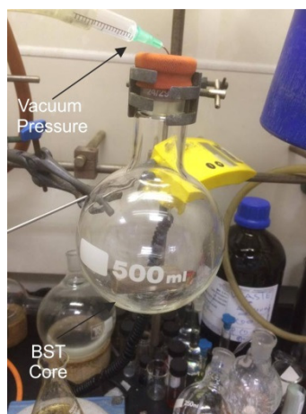
Figure 6.6: Saturation of BST core plug under vacuum pressure.
