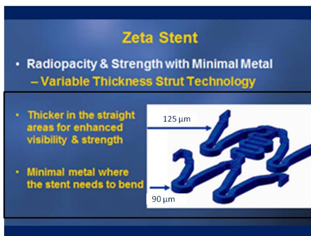
Figure 10. Variable thickness strut technology of the Multilink Zeta.
