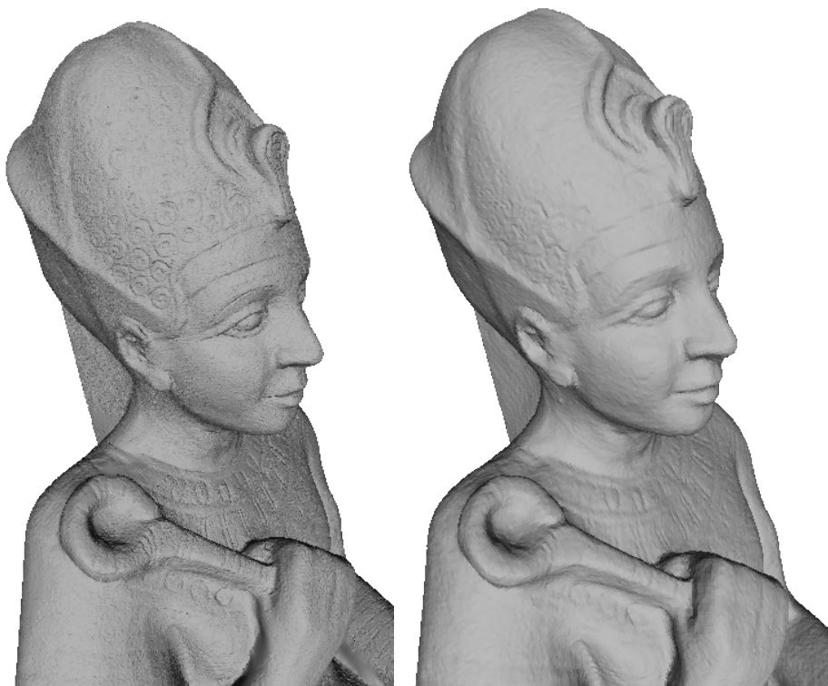
Fig. 4.7: Reconstruction from scan data. The mesh supplied from AIM@SHAPE is on the left, the layered reconstruction on the right.
