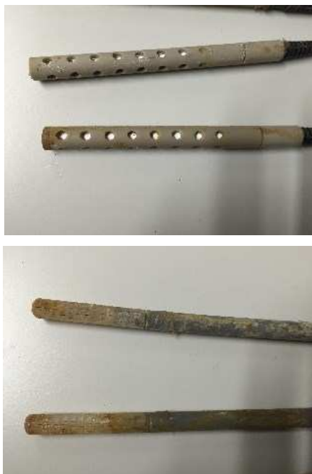
Fig. 5. Visible inspection of the PEEK (above) and epoxy (below) packaging after extended exposure in the sewer environment.
