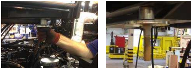
Figure 7. The crush-hand risk on the plant’s cab line – the original risk on left and its implemented resolution on right
