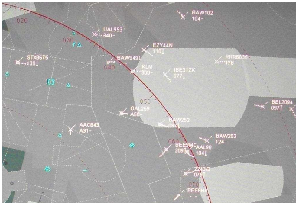
Figure 2: Example of colour coded data blocks used in air traffic control. Data blocks are clusters of small text containing descriptive information of a flight and altitude, the colour indicates whether they are owned or not and whether there are any warnings associated with a particular aircraft.
