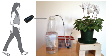
Figure 1: The Go & Grow system linking individuals' activity data to the amount of water that their personal plant receives.
