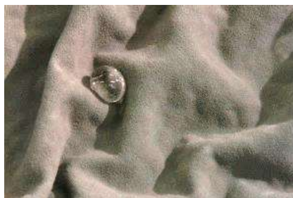
Figure A.1.1-6 Close up of the MycoCouture surface showing its hydrophobic properties (Park & Ivanova, 2013). Image courtesy of Dr Simon Park, 2013
