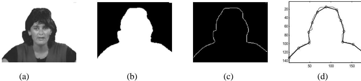
Figure 1: Shape coding example – (a) the 30 th frame of the Miss America sequence, (b) the segmented object shape, (c) the shape contour, and (d) shape coding – the solid line is the reconstructed contour using (lossy) encoded information, while the dotted line is the original contour (c).
