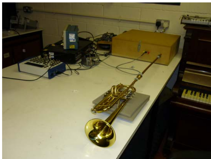
Figure 2 Acoustic pulse reflectometer coupled to trumpet
