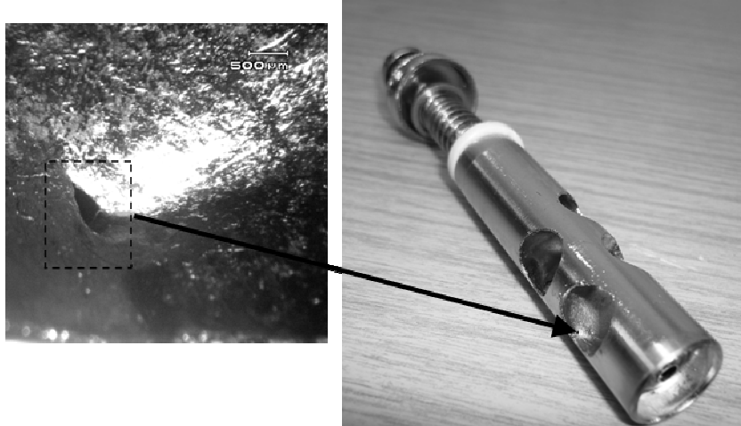
Figure 4 Third valve of trumpet B with leak in wall of lower channel.
