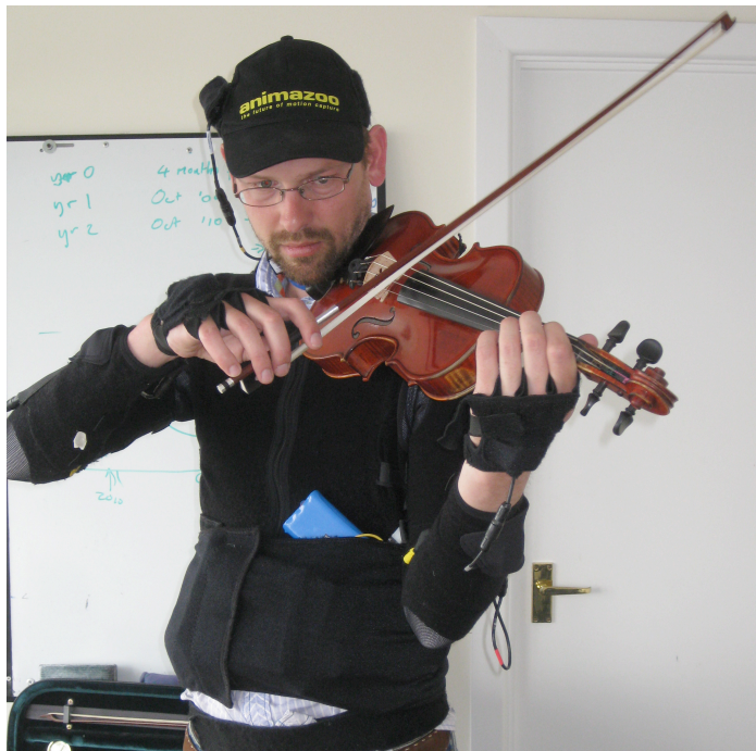
Fig. 3. A prototype of a motion capture and vibro-tactile feedback system for tracking and improving bowing actions when learning to play the violin [from 23]
