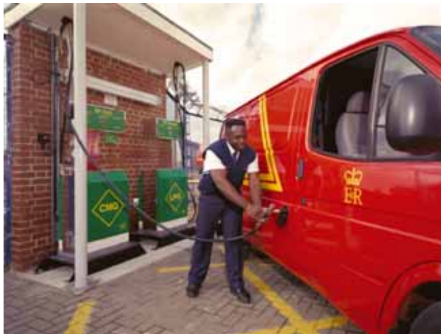
Figure 2.12 Refuelling a postal van in the UK with compressed natural gas, from a dedicated commercial vehicle at the Post Office's own site
