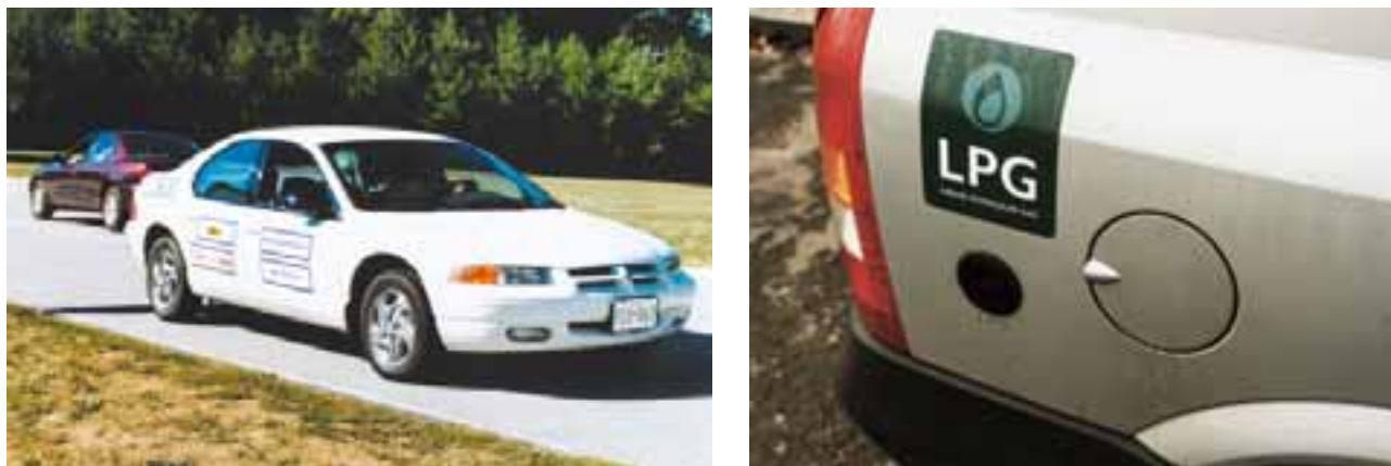
Figure 1.5 A vehicle powered by liquefied petroleum gas (LPG). Like CNG, LPG cuts local air pollution but CO 2 emissions are only marginally less than for conventional road fuels
