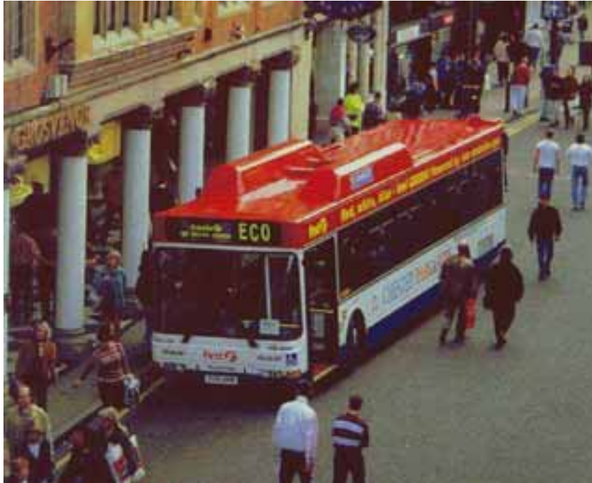
Figure 2.13 City bus running on LPG with fuel tanks clearly visible on the roof of the bus
