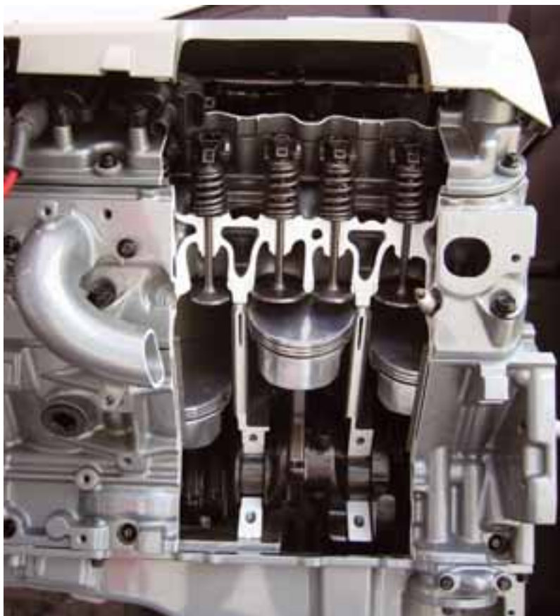
Figure 2.5 Cutaway of the Cadillac LS6 V8 injection engine
