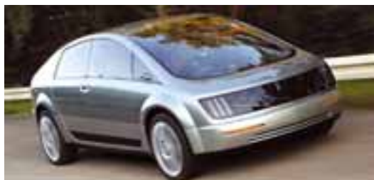
Figure 2.18 The General Motors concept car, Hy-Wire, is based on a platform module which contains a hydrogen-powered fuel cell along with complete replacement of traditional mechanical components by using drive-by-wire systems.
