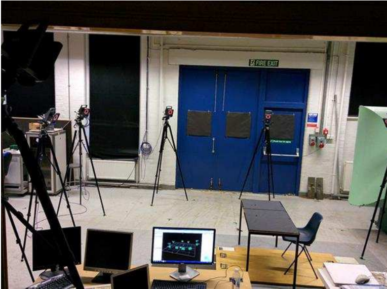
Figure 1: Ten-camera Vicon T-160 motion capture system
