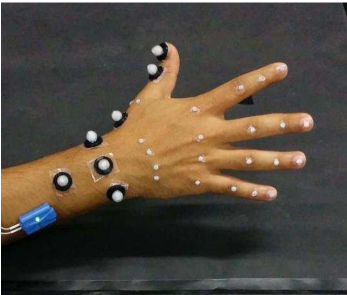
Figure 2: Marker positions for hand motion analysis
