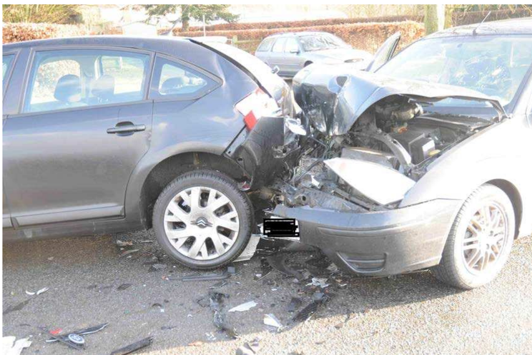
Figure 5.6(iv): Bonnet overlap & damage of Citroen [GP]
