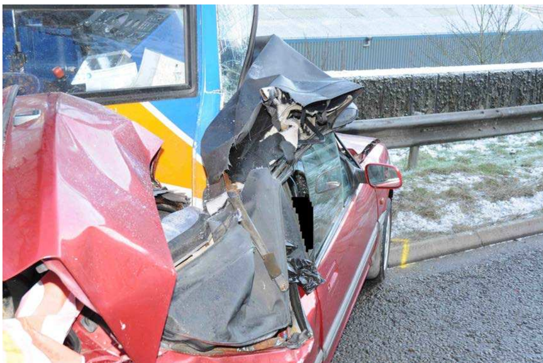
Figure 5.10(iv): Severe vehicle crush of Bus & Car bodies [GP]
