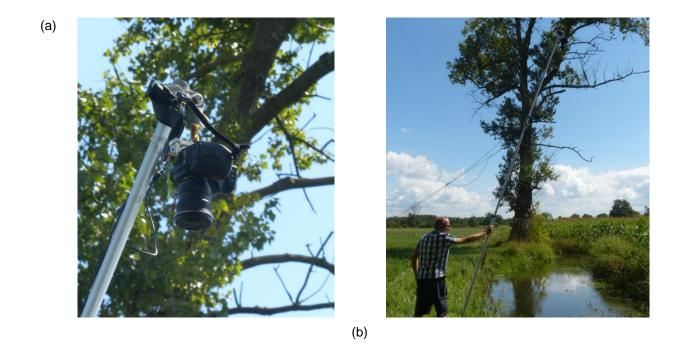
**Figure 2:** Illustrations of the image collection in the field. **(a)** The DSLR camera is attached with a ball head to a handheld telescopic pole to take orthogonal images. **(b)** One person holds the pole with camera tilted in order to position the camera at a height of 5 m above the water surface. A second person checks with a live view on a laptop that both river banks are visible on each image and takes the images with tethered capture.
