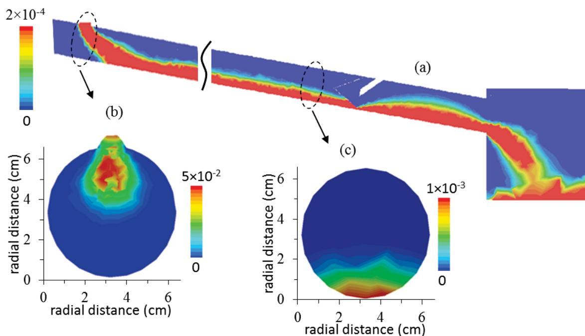
Figure 3. Solid (biomass) concentration (a) axial cross-section concentration profile over the entire simulation domain (concentration restricted to  $2 \times 10^{-4}$  to allow better visualization) (b) and (c) radial cross-section contour at the reactor entrance and 3.5 m from the entrance, respectively.
