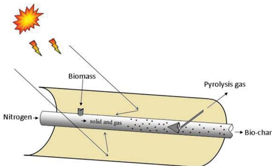
**Synopsis:** A model of biomass pyrolysis in a solar-thermal reactor is presented to show the potential of the concept for sustainable energy.
