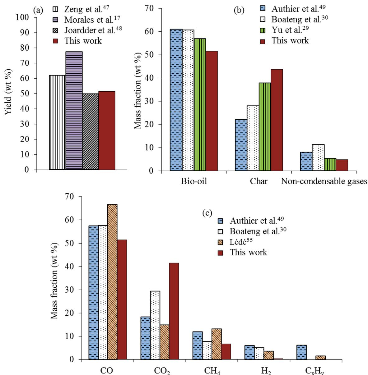
Figure 9. Products composition in comparison with the literature data (a) Bio-oil yield compared to literature data obtained in solar reactors (b) mass composition of the overall product compared to the wider literature data (c) mass composition of the non-condensable gas in comparison to the literature data. Details of reactors and operating conditions are given in the supporting information (Table S2).
