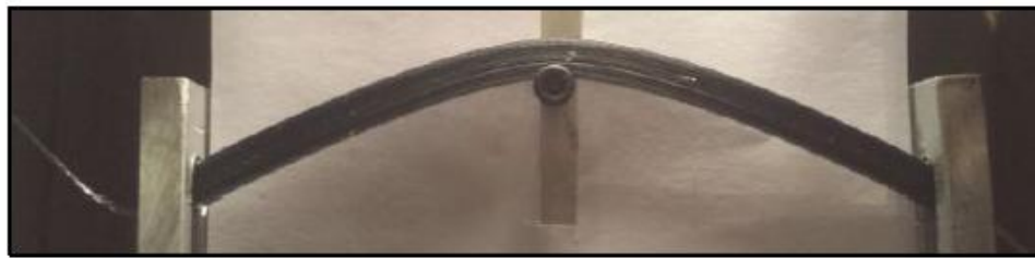
Figure 2. Bend test on the 3D printing embedded structure. The fibre is embedded near the neutral axis of the fibre
