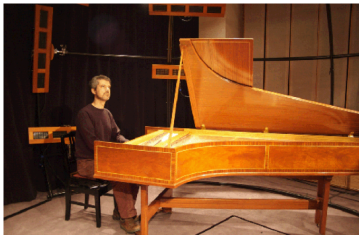
FIGURE 6.3: Image of the interactive auralisation system developed by Woszczyk. The sound from the musician is picked up by a directional microphone and convolved with a 24-channel room impulse response. The room response is rendered over a 3D loudspeaker array which is visible behind and to the left of the musician. Impulse responses were measured using an array of 8 directional microphones positioned at 3 different heights. Image reproduced from Woszczyk and Martens (2008)
