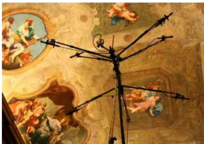
FIGURE 3.8: Microphone array utilised by Woszczyk et al to record spatial impulse responses of different performance spaces. This microphone array consists of eight microphones arranged in identical directions to a loudspeaker array. In this particular measurement system, impulse responses were captured with the microphones at three different heights in order to feed a 24-channel loudspeaker array. Reproduced from (Woszczyk et al., 2012)
