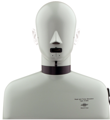
FIGURE 3.6: Image showing a Brüel Kjør 4128C - Head and Torso Simulator (HATS) (Brüel & Kjør, No date). The dummy head features microphone capsules arranged behind latex pinnae allowing binaural impulse responses to be recorded. This system also features a loudspeaker in the mouth of the dummy in order to measure Oral-Binaural Room Impulse Responses as demonstrated by Cabrera et al. (2013)
