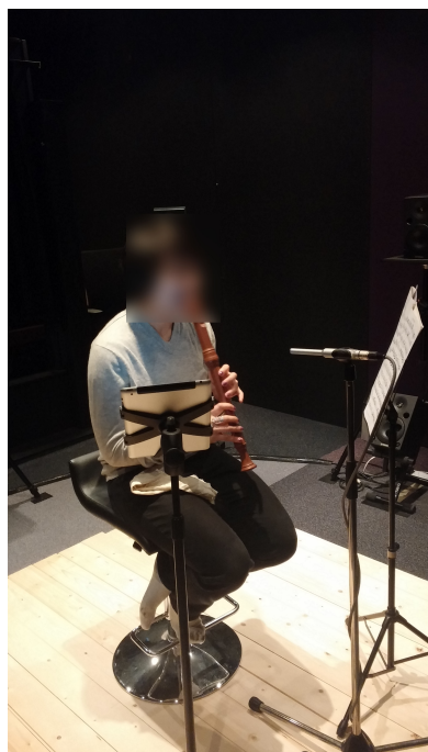
FIGURE 8.2: Photo showing the position of the microphone relative to a musician playing in the interactive auralisation system. The microphone is positioned directly in front of the musician at a radius of 30cm and a height of 1m from the floor. Also positioned around the musician are an iPad interface and a music stand.
