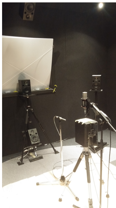
FIGURE 8.10: Measurement system positioned in the sweetspot of the loudspeaker array. A Genelec 1029A loudspeaker is mounted at a height of 0.93m (floor- top of LF driver height) and the Soundfield ST350 ambisonic microphone is mounted at a height of 1.29m above the wooden floor. The sound from the loudspeaker is captured by a Behringer ECM1000 omnidirectional measurement microphone positioned 30cm from the measurement loudspeaker. Absorption was applied to the LCD screen and a wooden floor deployed
