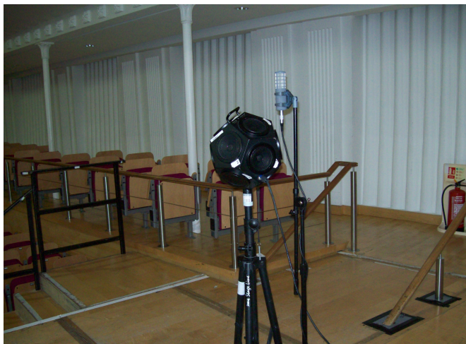
FIGURE 3.17: Image showing the relative positions of the dodecahedron loudspeaker and sound-field microphone.
