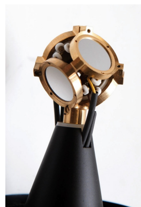
(b) Tetrahedral arrangement of microphone capsules in an Ambisonic microphone (Studiocare, No date)
