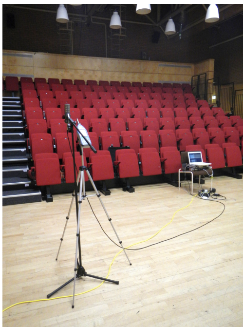
FIGURE 3.19: Image showing the relative positions of the Ambisonic microphone and sound level meter for background noise measurement in the Ledger Recital Room.
