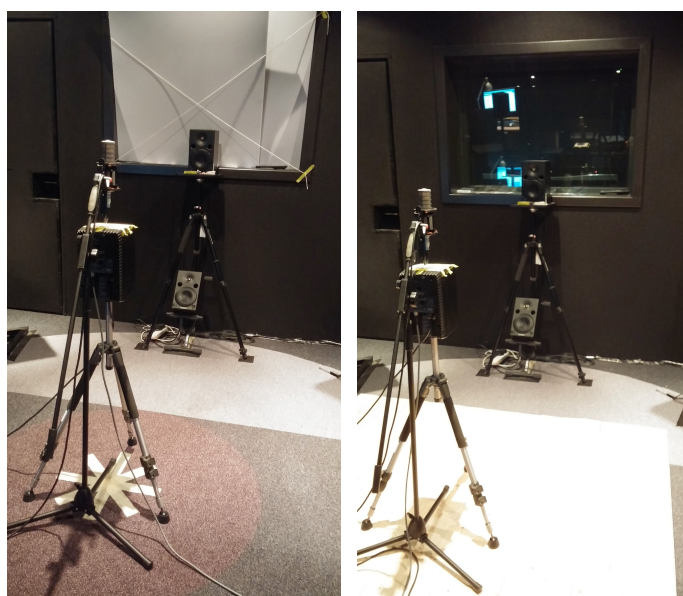
(a) Without floor - With Screen absorption (b) With floor - Without Screen absorption
