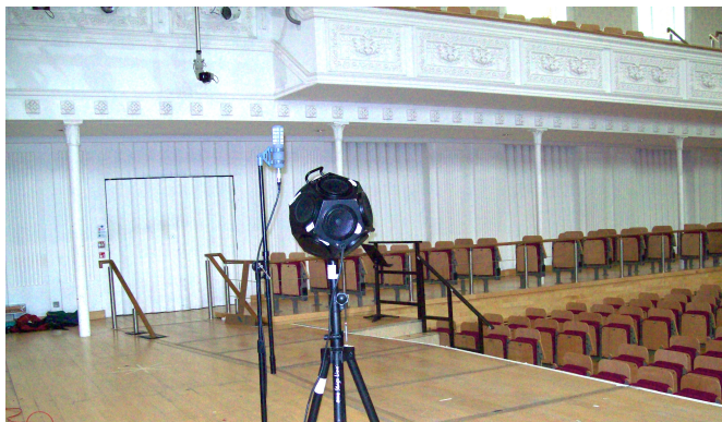
FIGURE 3.13: Image showing the relative positions of the dodecahedron loudspeaker and sound-field microphone.
