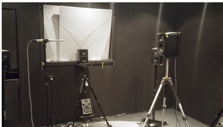
FIGURE A.1: Image showing the relative positions of the loudspeaker and microphone. The radius between the transducers was 1m. The other loudspeakers shown in the image were not used in the experiment. The loudspeaker was rotated in 10^\circ increments after each measurement.
