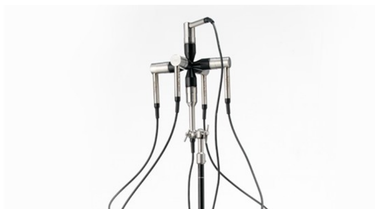
FIGURE 3.12: Image showing a G.R.A.S. 50VI-1 Vector intensity probe consisting of 6 omnidirectional microphone capsules. Reproduced from (G.R.A.S. Sound Vibration , 2013)
