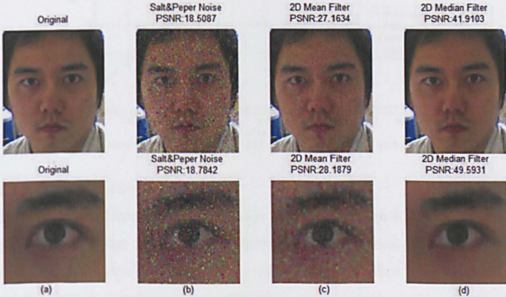
Figure 3.3 Comparison of image smoothing methods (a) Original image; (b) Polluted image with ‘salt & pepper’ noise; (c) Result of applying mean filter; (d) Result of applying median filter
