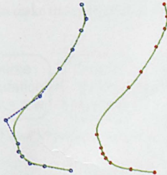
Figure 5.7 NURBS curve by reverse computation circles (blue) represents the computed control points dots (red) represents the original data points
