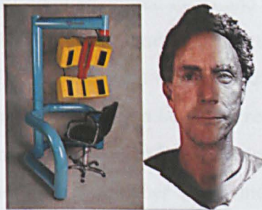
Figure 2.5 Cyberware 3D face and face system Left: 3D scanner; Right: sample scanned data with more than 1,400,000 polygons
