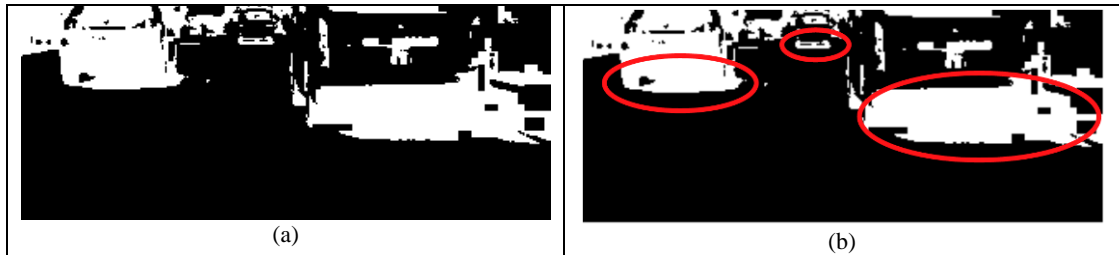
Figure 4-19: (a) Binary image with white colour representing the area that is darker than the minimum grey-level of the identified road region. (b) Multiple regions for potential vehicle detection, circled in red colour.
