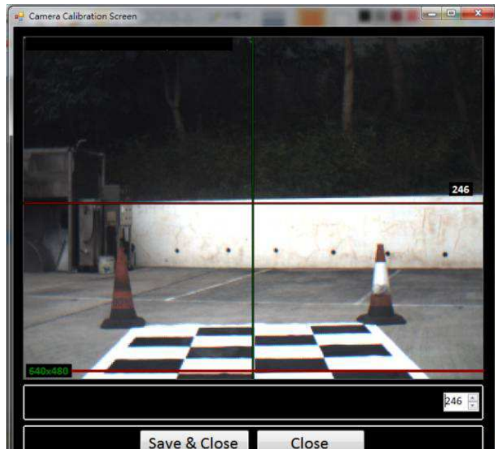
Figure 4-2: Captured image with aligned horizontal and vertical line. The roll and pitch angles are almost zero.
