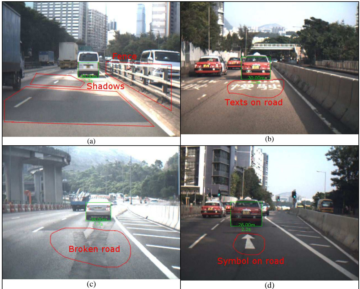
Figure 4-9: Challenges appeared in the test video sequences. (a) Road-side fence and shadows. (b) Texts on the road. (c) Broken road. (d) Symbol on the road.
