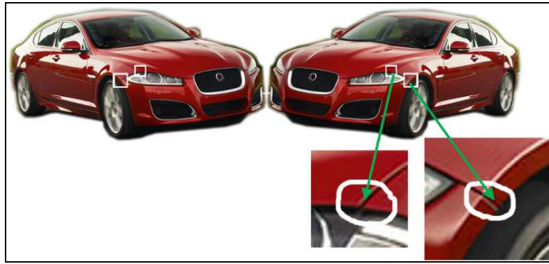
Figure 3-8: Illustration of good symmetric positions for symmetric geometrical line construction for camera calibration. The square boxes shown on the left and right side of the vehicle indicate example locations for good symmetrical geometrical line construction.
