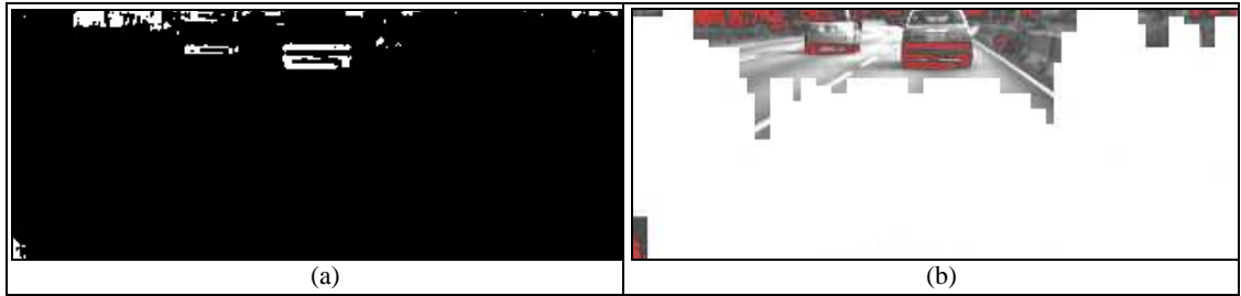
Figure 3-26: (a) Binary image with those white areas representing regions that are darker than the minimum graylevel of the road region. (b) Binary image in (a) overlaid to the ROI of the captured image. Those horizontal contours along the rear part of vehicles at the front are identified.
