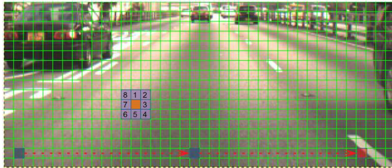
Figure 3-18: Captured image showing 16x16 grid lines in green colour. The seed block is searched from the bottom left to the bottom right of the image until a block is found with satisfactory mean and standard deviation. An example block highlighted in orange colour is compared to its neighbour blocks marked with number 1 to 8 with purple colour.
