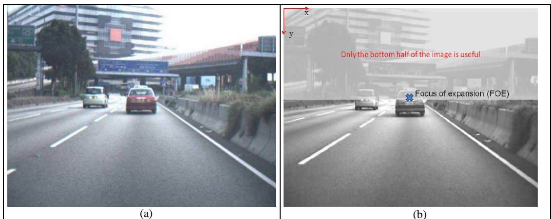
Figure 3-21: (a) Typical captured image that has been converted to grayscale image. (b) The FOE and the primary ROI is selected as the area below the FOE.
