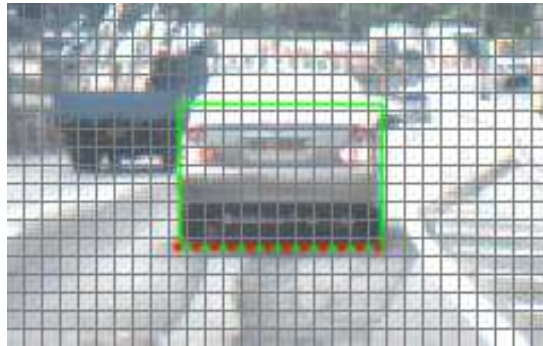
Figure 3-34: Speed measurement based on binning of the MVs along the bottom line of the rectangle bracketing the detecting vehicle. Red dots in the image indicate the MV samples for true ground speed evaluation.
