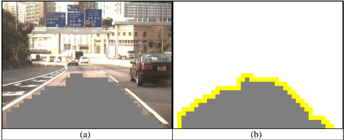
Figure 7-2: Road region identified in a captured frame and the corresponding diminished road region for use in the next frame. (a) Captured frame with identified road region. The identified road region is shaded with grey colour blocks. (b) Extracted road region from (a). The boundary is diminished by 1 block along the contour. The yellow contour is the difference between the original and diminished contours.
