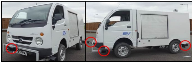
Fig. 2. Tata ACE autonomous vehicle platform showing LIDAR sensors.
