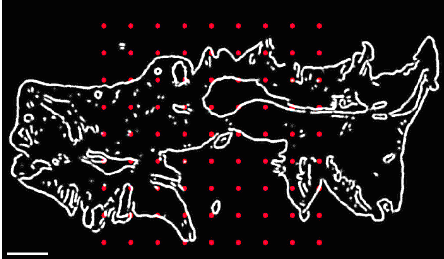
Figure 2.13: The centres of rotation used for rigid slide registration. Each point shown in red is used as a centre of rotation for the algorithm. The size and spacing of this grid varied depending on the transformation step. Scale bar represents 5 mm.
