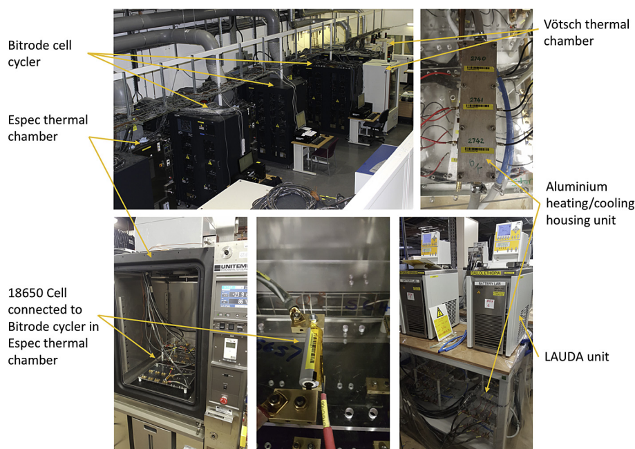
Fig. 2. Pictures showing the experimental set up for long term ageing tests at WMG's Energy Innovation Centre.
