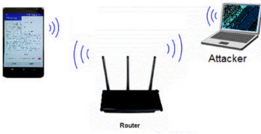
Fig. 1: Attack environment for network denial of service consists of an Android phone, a laptop and a wireless router
