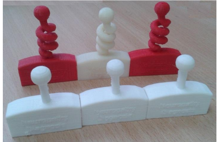
Fig. 3. The range of 3D printed phone attachments.
