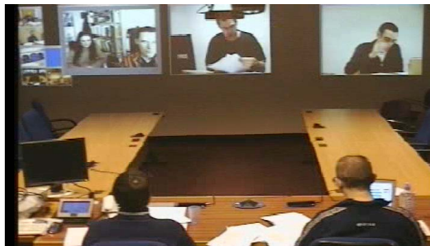
Figure 1: View of an AG Node, a designed room intended for end-users to ‘walk in and meet over videoconference’. Three projectors are aligned to show large format video, remote controlled cameras provide participant closeup and whole scene images, and full-duplex microphones are arranged on the tables.
