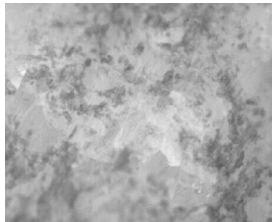
Figure 4. Detection of fluorescence using the UV LED. The image is a difference image between an image acquired without any illumination LED's and an image with the UV led switched on. The bright regions corresponds fluorescence in the rock surface.
