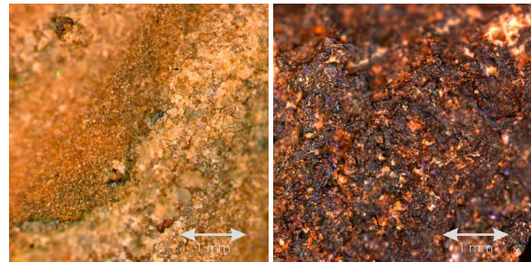
Figure 2: Microscope images from a layered limestone (left) and a basaltic volcanic rock (right).
