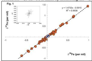
signal and applying an on-line mathematical correction at mass 54. Blank subtraction is undertaken off-line. The effect of <sup>40</sup>Ar<sup>16</sup>OH background at mass 57 is reduced by analyzing solutions at approximately 10ppm concentration and sample and standard solutions are concentration matched to within 5%. Typical errors are less than 0.05 per mil (2 sigma) in most cases.
