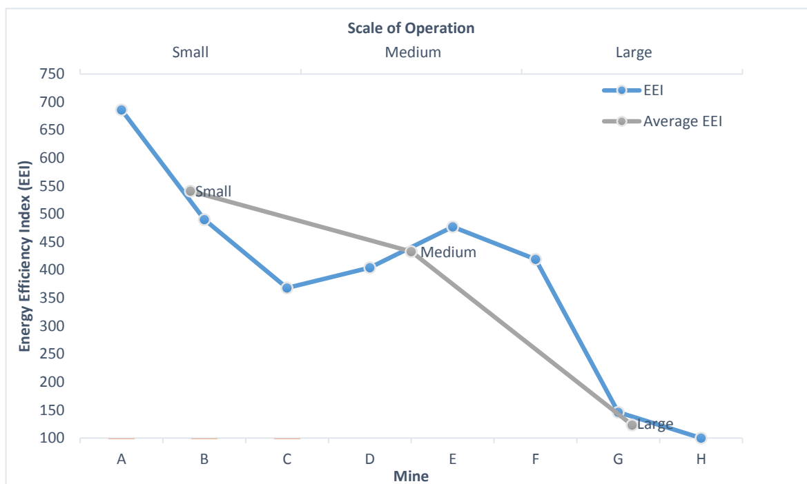
Figure 3.2: Energy efficiency index for iron ore mines and the average energy efficiency index for small, medium and large iron ore mining operations in Western Australia
