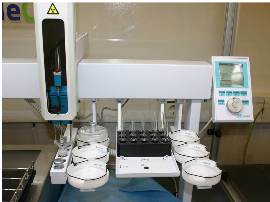
Figure 1: Ampoules filling station of the automatic dispensing robot.
