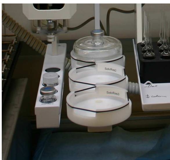
Figure 3: Solvent reservoirs and wash and waste vials with closed septa.
