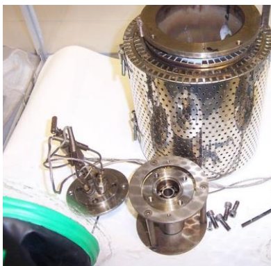
Fig. 1. Vessel (front) and furnace (back, insulation removed) for water sorption studies.
