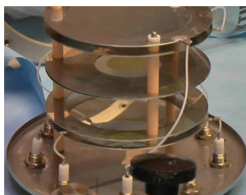
Figure 15 Gridded ionisation chamber with a ^{242}\text{Pu} target in the centre as cathode for measurements of ^{242}\text{Pu}(n,f) cross sections versus ^{238}\text{U}(n,f) at IRMM xvi
