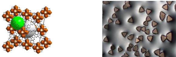
Figure 1 : View of the structure (left) and optical microscope picture (right) of [\text{Np}_6\text{O}_4(\text{OH})_4\text{L}_6(\text{H}_2\text{O})_6]
