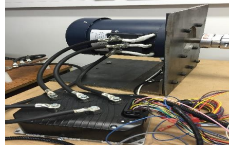
Fig. 9. Inverter (motor controller) and 14kW AC motor
