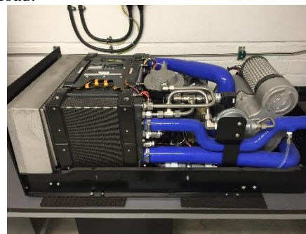
Fig. 3. 8.5kW PEM Fuel Cell test platform
