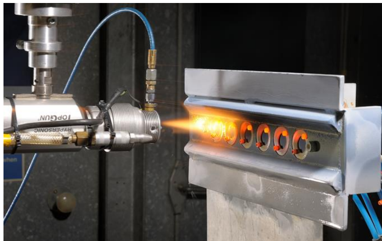
Figure 14 Photograph showing the large thermal load experienced by the substrate and jigging from the passing HVSFS torch as seen by the glowing mounting rings. This photograph is taken from related trials using alcoholic titania suspensions with comparable flame conditions.
