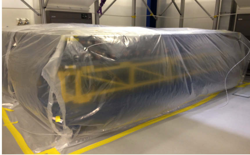
Figure 7.11: Photograph of the anti-radon tent covering the C-section.
