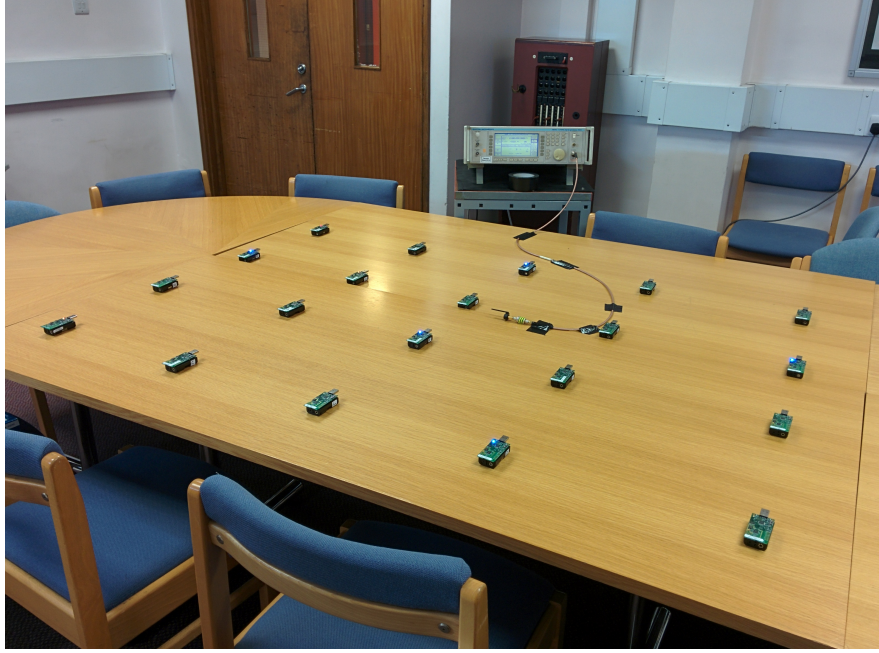
Figure 5.11: Example of one of the four rooms comprising an experimental setup. The four right-most nodes in the image are used for noninvasive network observation, while the RF signal generator, which acts to generate interference, is shown in the background.
