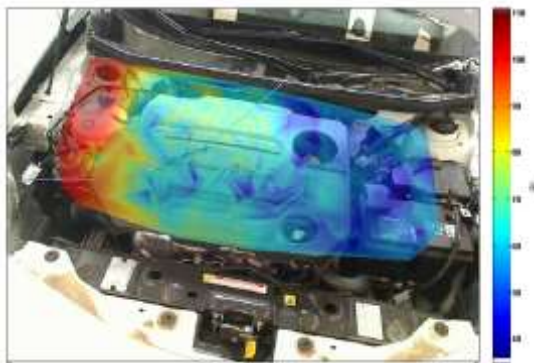
Fig. 17: Acoustic map of particle velocity at 49.8 Hz (1500 rpm with cover presence)
