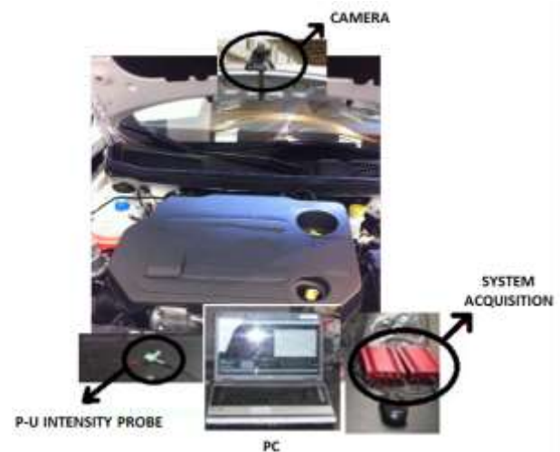
Fig. 7: Experimental setup of near field measurements
