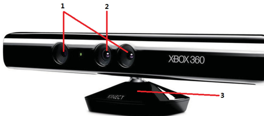
Figure 3. Image of Kinect sensor: 1. Depth sensors, 2. RGB camera, 3. Motorized base. Modified from Reddivari et al. (2014).
