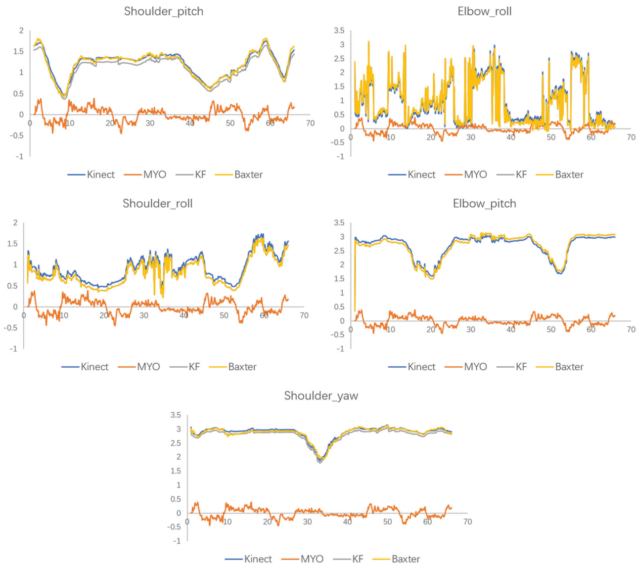
Figure 13. Graphical result after the Kalman Filter-based sensor fusion ( Shoulder Pitch, Shoulder Roll, Shoulder Yaw, Elbow Pitch, Elbow Roll).
